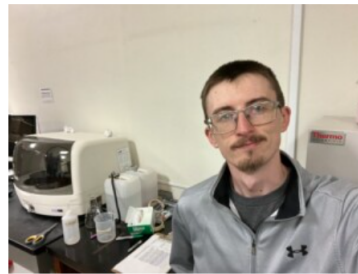
Corbin Kohart, Northwest Coastal Inland Base Crew Lab Coordinator, stands by the AQ2 discrete analyzer, which measures nutrient content from H2Ohio Wetland soils and water samples.
